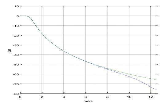
Figure 5. Discrete-time (blue) and continuous-time (green) frequency responses note:  $f_s/2 = 2$  Hz = 12.57 rad/s
