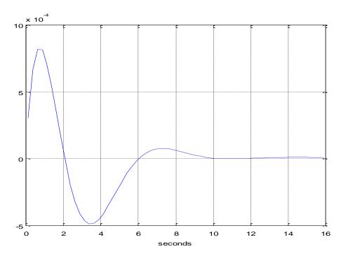
Figure 4. Error of discrete-time step response
