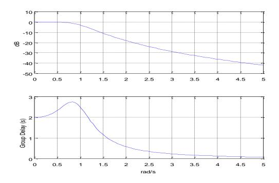
Figure 5. Frequency Response and Group Delay of the discrete-time filter.
