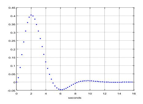
Figure 1. Impulse Response of discrete-time 3<sup>rd</sup> order Butterworth Filter
